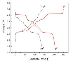
Fig. 1 Charge/discharge curves of O3-NiMn in 1.5 - 4.5 V at 1st and 10th cycle.
