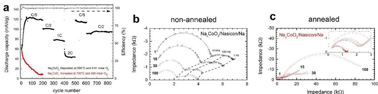
Fig. 1a, discharge capacity and efficiency of  $\text{P2-Na}_x\text{CoO}_2/\text{Nasicon}/\text{Na}$  batteries with as-grown (black) and annealed (red)  $\text{P2-Na}_x\text{CoO}_2$  cathode at the cycling rates between C/5 and 2C. Impedance spectra of a  $\text{P2-Na}_x\text{CoO}_2/\text{Nasicon}/\text{Na}$  battery with (b) not-annealed and (c) annealed cathode between 1 and 100 cycles.
