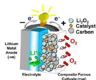
Fig.1 Schematic representation of a rechargeable Li-air battery.
