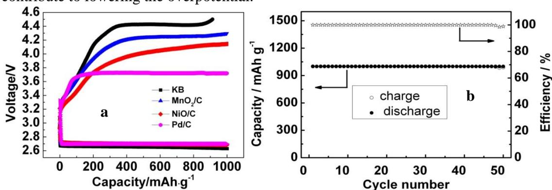
Figure 2. (a) Comparison of the first discharge-charge curves of the Ketjen black, MnO<sub>2</sub>/C, NiO/C, and Pd/C at 0.1 mA cm<sup>-2</sup>, with a capacity limited to 1000 mAh g<sup>-1</sup> (b) Comparison of the cycling performances of Pd@C macroporous electrode.
