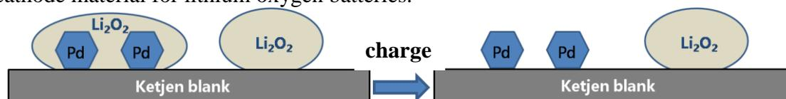
Figure1. Schematic of the nanostructured cathode architecture. This figure shows the the palladium nanoparticles and the nanocrystalline lithium peroxide, all of which contribute to lowering the overpotential.
