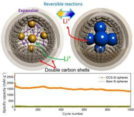
Double carbon shell-encapsulated Si nanoparticles (DCS-Si) perform dual functions, which deliver a high reversible capacity of 1802 mAh  $g^{-1}$  at 0.2 C, superior rate capability, and cyclability (1000
