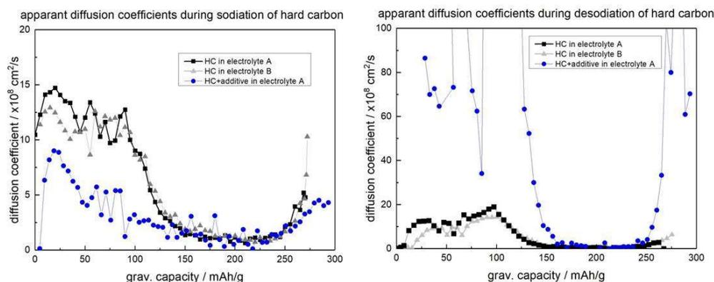
Fig 1. Apparent diffusion coefficients during sodiation (left) and desodiation (right) for three different test cells; black squares: standard HC electrode in electrolyte A; grey triangles: standard HC electrode in electrolyte B; blue circles: HC electrode comprising an ionic conductor in electrolyte A.
