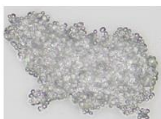
Figure 1 A snapshot of fine particles without electrolyte solution
