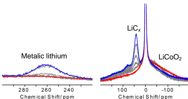
**Fig. 1.** *In situ*  $^7\text{Li}$  NMR spectra observed at  $0^\circ\text{C}$  with the charging rate of 1 C during the charging process. Red and blue lines correspond to the first and the last spectrum, respectively.
