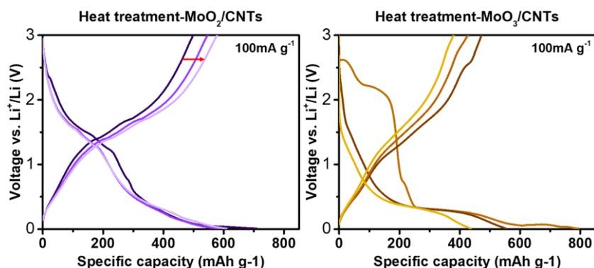
**Figure.** Discharge and charge curve of MoO<sub>2</sub>/CNTs and MoO<sub>3</sub>/CNTs composite
