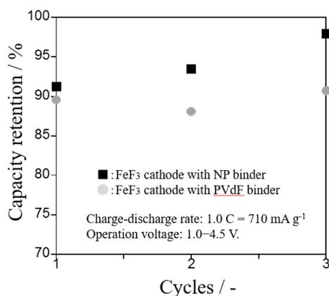
Figure 1 Cycle performances (Charge capacity) of Li-metal half cells composed of  $\text{FeF}_3/\text{AB}$  with (■) NP binder, (●) PVdF binder.
