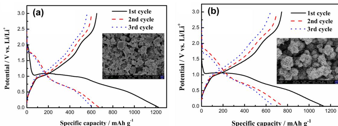
Fig. 1 Lithiation/de-lithiation curves and SEM micrographs of (a) eMCMB electrode and (b) eMCMB electrode with modified nickel oxide nanoflakes.
