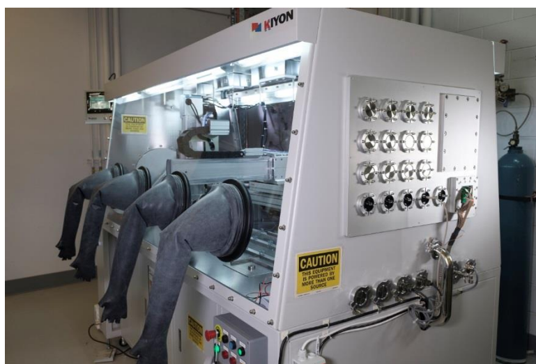
Figure 1 – The high throughput robotic electrochemical testing system (FASTER).
