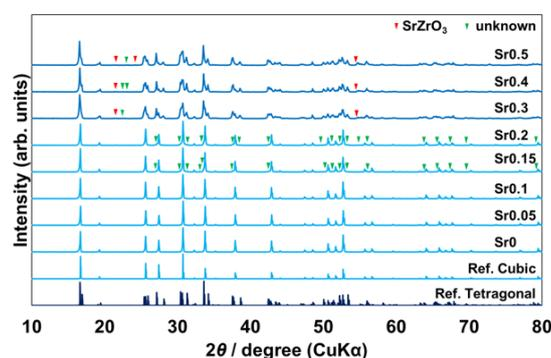
Fig. 1 XRD patterns for  $\text{Li}_{6.25+x}\text{Ga}_{0.25}\text{La}_{3-x}\text{Sr}_x\text{Zr}_2\text{O}_{12}$  synthesized at 1000 °C for 12 h in air.
